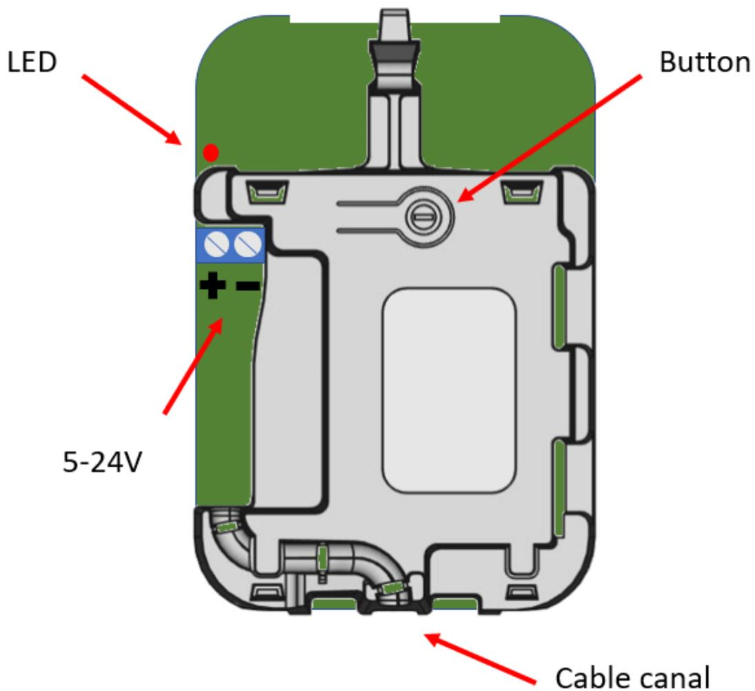
Configure the device in the LoRaWAN server, according to chapter 5.1, and power the device with 5-24 VDC power, e.g. USB charger or 24 VDC. The cable can be routed through the cable canal or through the electronic board for junction box mount. The sensor starts and flashes 8 times during the boot-up sequence and starts the join sequence to the LoRaWAN network
