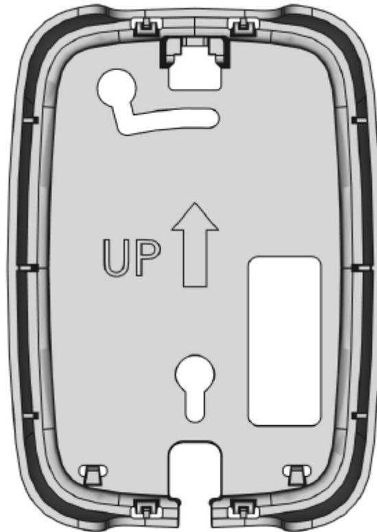
The bottom piece is mounted on the wall with the “UP” arrow upwards. It can be mounted either with screws or adhesive tape both included in the package. The hole pattern matches standard junction box.
